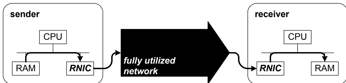
(b) Thanks to the direct data placement mechanism provided by RDMA-enabled NICs (RNIC), the network can be fully utilized with minimal overhead on the end-hosts.
